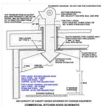
**508.4** Construction of Type II Hoods. Shall be constructed of steel not less than 0.024 (No 24MSG) of an inch in thickness. Hoods constructed of copper shall be of copper sheets weighing not less than 0.17 ounces per square inch. Joints and seams shall be substantially tight. Solder shall not be used except for sealing a joint or seam.
