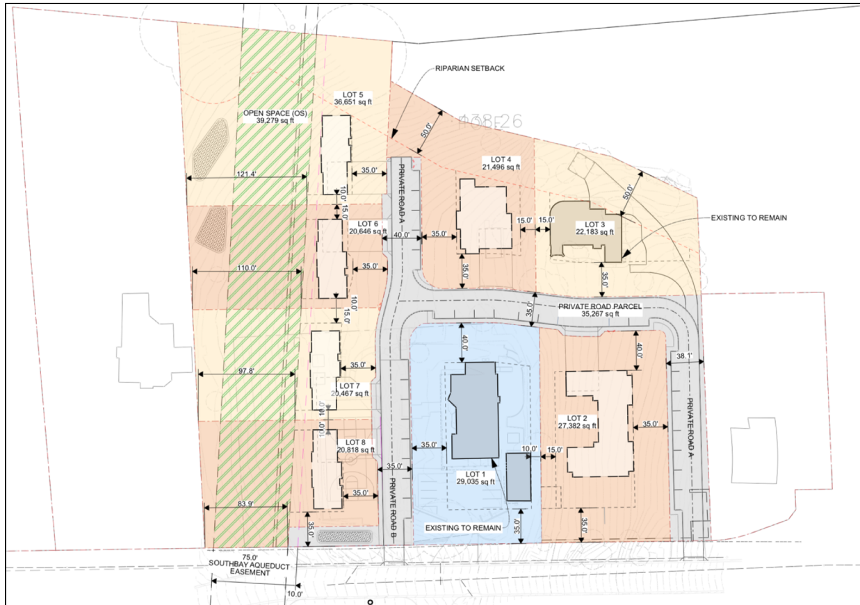
Figure 2: Site plan showing all the proposed development and subdivision of the adjacent three parcels to create eight separate parcels for potential construction of six new single-family houses, and a private road parcel.
