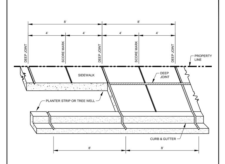
DEEP JOINT: DEPTH EQUAL TO 1/4 OR MORE OF SLAB THICKNESS. FINISH WIDTH AT THE TOP TO BE 1/2" MAXIMUM.
