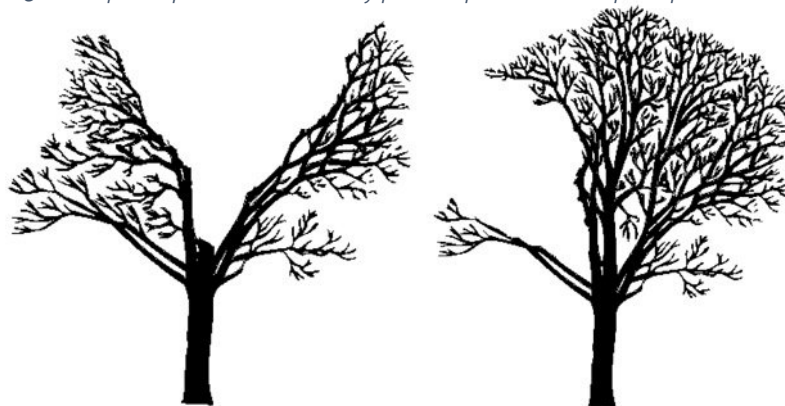
Figure 13. Examples of trees directionally pruned for clearance from power lines
