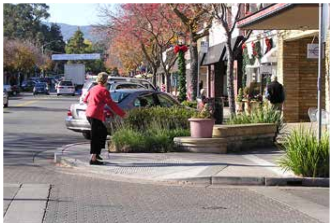
A bulbout reduces pedestrian crossing distances, slows turning cars, and provides a place for landscape and street furniture.
