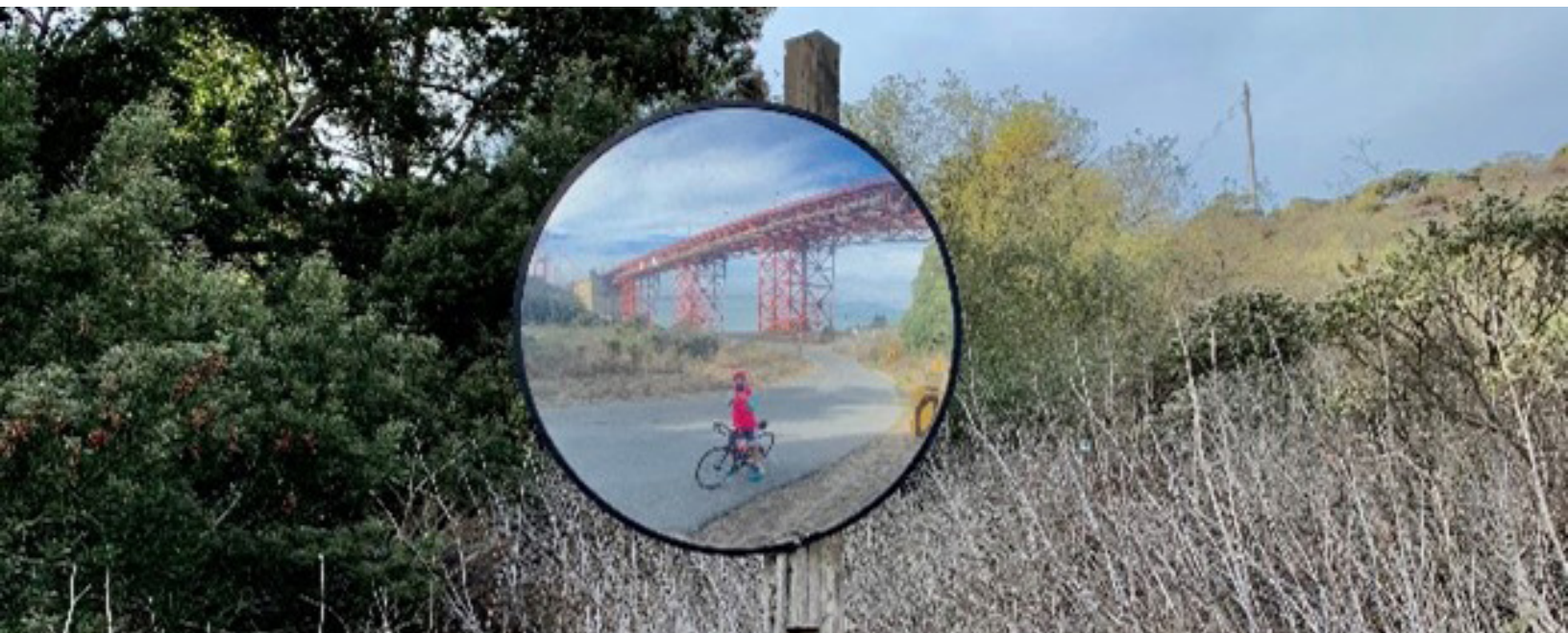
Trail mirror at path under the Golden Gate Bridge provides additional safety where adequate sight lines are not possible.
