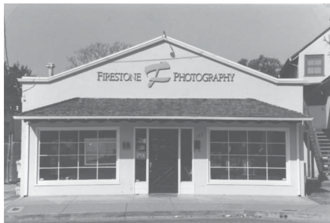
Figure 28. This commercial building on Washington Boulevard has generous display windows with multiple panes, clear signage, and an awning-like roof that gives weather protection and shade to pedestrians.
